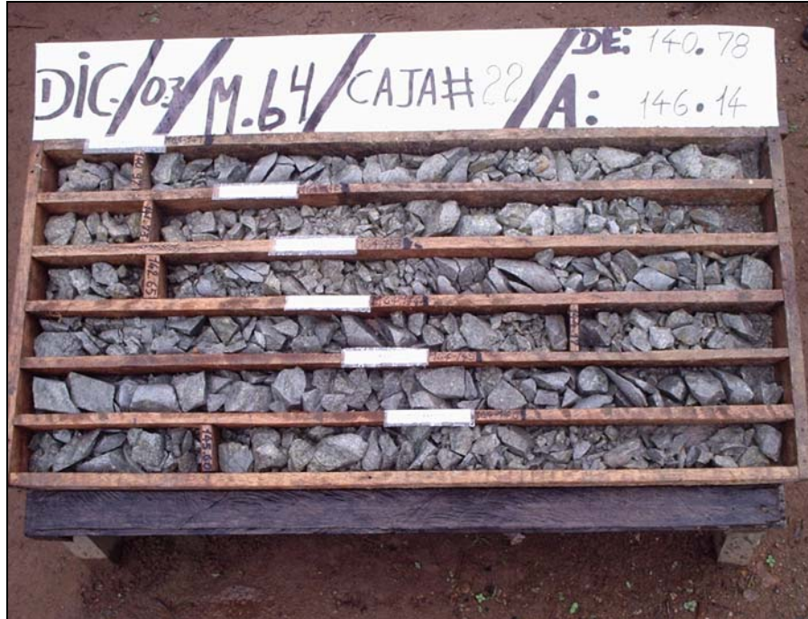
Figure 3-1: Drill Core Photo of M64 from 140.78 to 146.14 m showing Low RQD prior to Core Cutting
