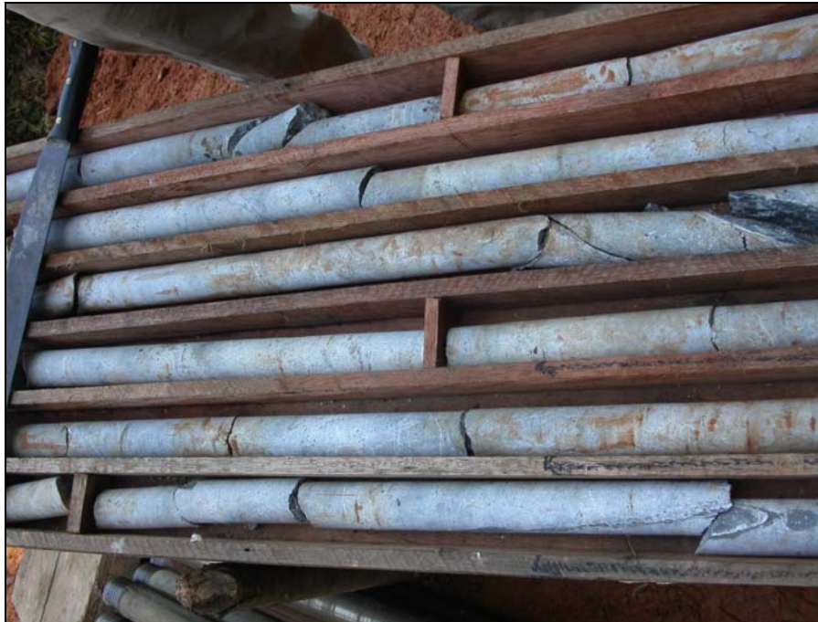
Figure 3-2: Drill Core with Unaltered Anhydrite (Below the Gypsum Front)
